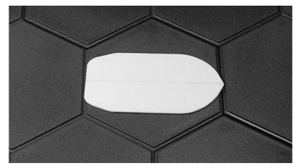
A second oblong of Plasticard is then cut out. This should be slightly larger than the original oblong as this will make the laminating process easier.
