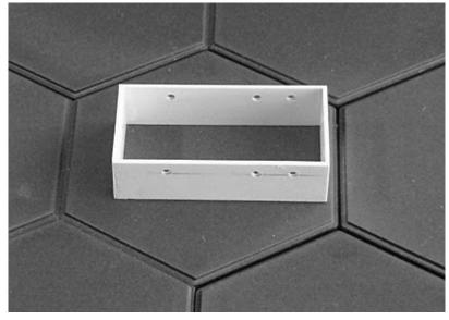
The 'lid' of the box can then be cut and glued in place and gently weighed down whilst the glue cures.
