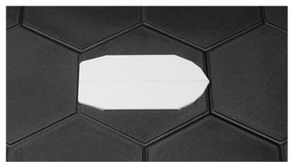
N.B. I use a Stanley knife/box cutter with a sharp blade to do the cutting, and it is done on a special non-slip rubber modelling mat. A ruler with a non-slip surface is used to cut any straight edges. <u>I strongly recommend that anyone following this method use similar</u> tools at all times when cutting the Plasticard as it will make the whole process much safer and more accurate.
